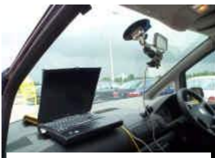
Car mounted GIS/GPS video surveys
